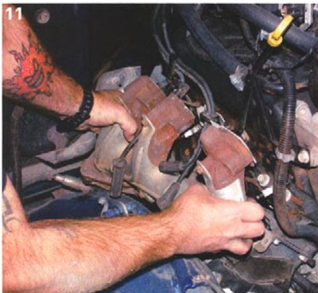
Once the bolts were off, the manifolds were removed.
