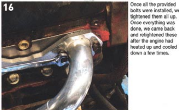
Now the shorty headers were slipped right in. JBA did such extensive R&D on these pipes that they had a factory fit; nothing hit or had to be massaged with a ball peen.
