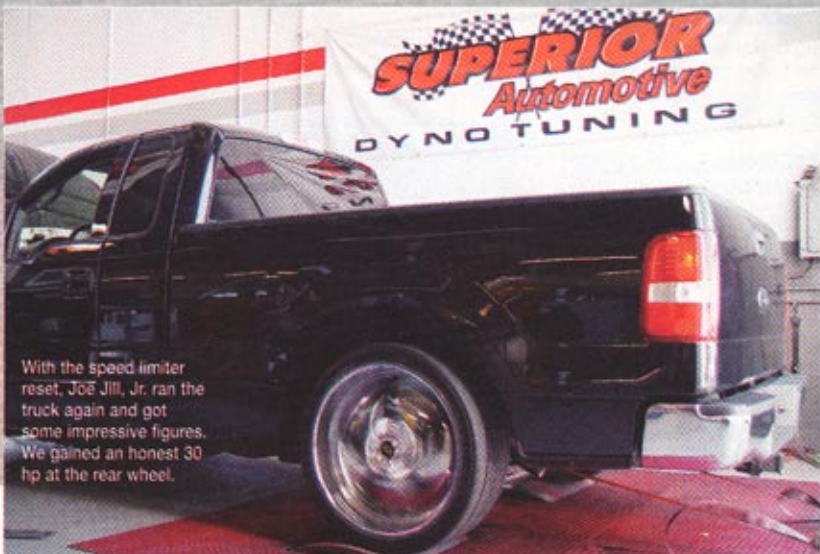
Shawn Ellis of SoCal Tuning & Performance used a Predator plug-in tuner from DiabloSport to set the speed limiter to 120 mph for our dyno runs.
