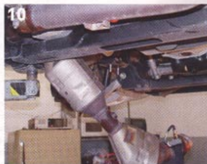
The driver-side front exhaust section was then unbolted from the manifold and the crossover pipe.
