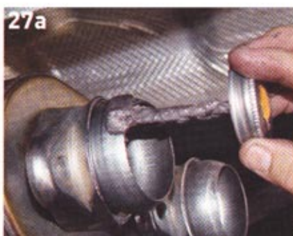
Then, after applying anti-seize compound to the ball and socket connector, the tips were bolted to the muffler, and the new hangers were connected.
