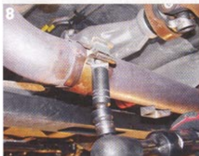
The back end of the exhaust manifold pipe was then unbolted.
