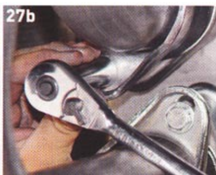
Then, after applying anti-seize compound to the ball and socket connector, the tips were bolted to the muffler, and the new hangers were connected.
