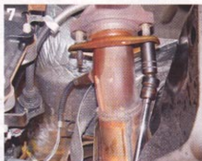
Starting on the passenger side, the nuts attaching the manifold to the exhaust were removed.
