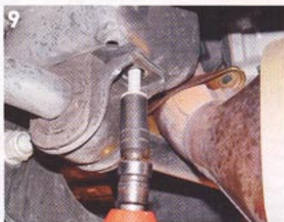
The sway bar was also unbolted and removed for extra clearance.
