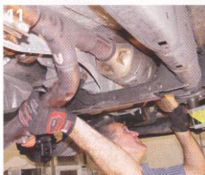
Then the passenger-side front exhaust section was removed.
