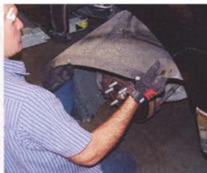
Then, with the engine cool and the truck on a lift, Ed Howard began by removing the inner fender panels for easier access to the exhaust manifolds.
