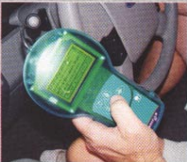
Shawn Ellis of SoCal Tuning & Performance used a Predator plug-in tuner from DiabloSport to set the speed limiter to 120 mph for our dyno runs.
