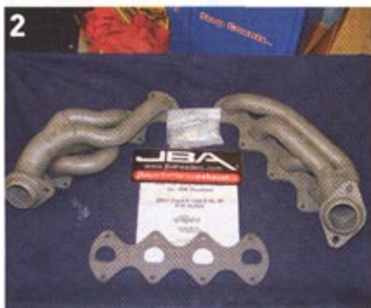
We installed a set of legal, stainless steel JBA Cat4ward headers with the optional high-temp JBA Titanium ceramic coating.
