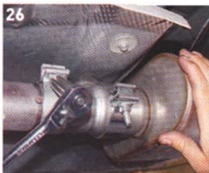
The muffler was then connected to the cat pipe using Bassani's supplied stainless steel fasteners.
