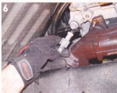
Then, all oxygen sensors were unplugged or unbolted from the exhaust.
